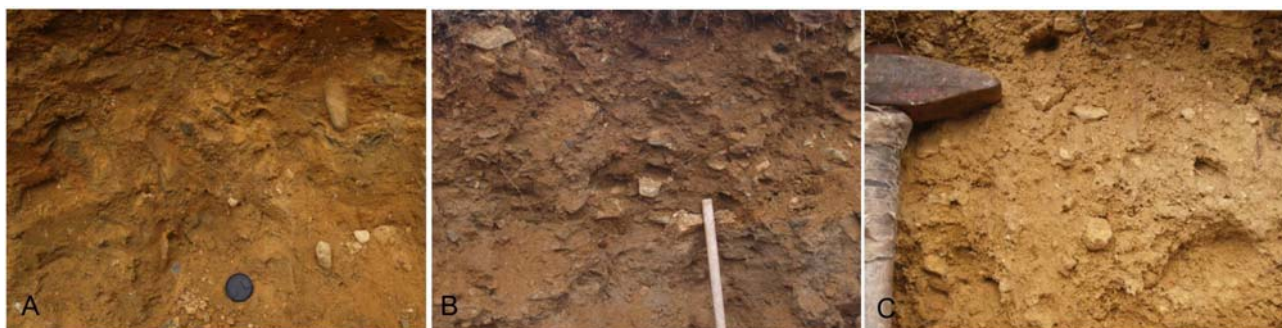
Figure 3. Images of soils in sluicing sites of Lapland gold rush areas. A) Clayey unsorted till at Suolaoja, Ivalojoiki area. Note the red and yellowish brown shades of the soil due to the abundant lateritic material and absence of sorting. B) Poorly washed clayey till at Ellioja, upper course of Palsioja, Ivalojoiki area. Oriented boulders indicate SW transport of the drift. C) Clayey unsorted till at the river bank, lower course of Palsioja, Ivalojoiki area.
