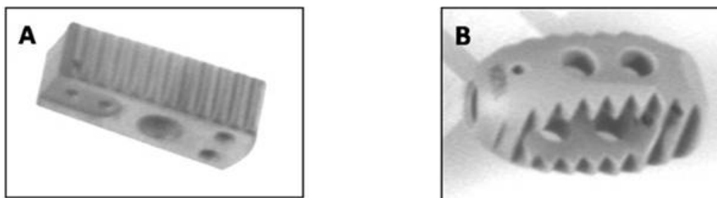
Fig. 1. Images of the two distinct cages, which biomaterials are composed of carbon fibre reinforced polymer (CFRP) (A) and polyetheretherketone (PEEK) (B), respectively.
