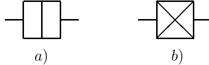
Figure 2.2: Symbol for a a) normal metal tunnel junction and b) superconducting tunnel junction.
