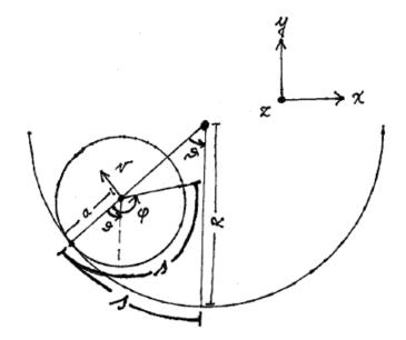
The total kinetic energy consists of the kinetic energy for the c.m (center of mass) and the kinetic energy related to the rotation around the c.m
