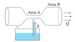
where  $v_b$  and  $v_a$  are velocities of flow in parts of the construction at area B and area A, respectively.
